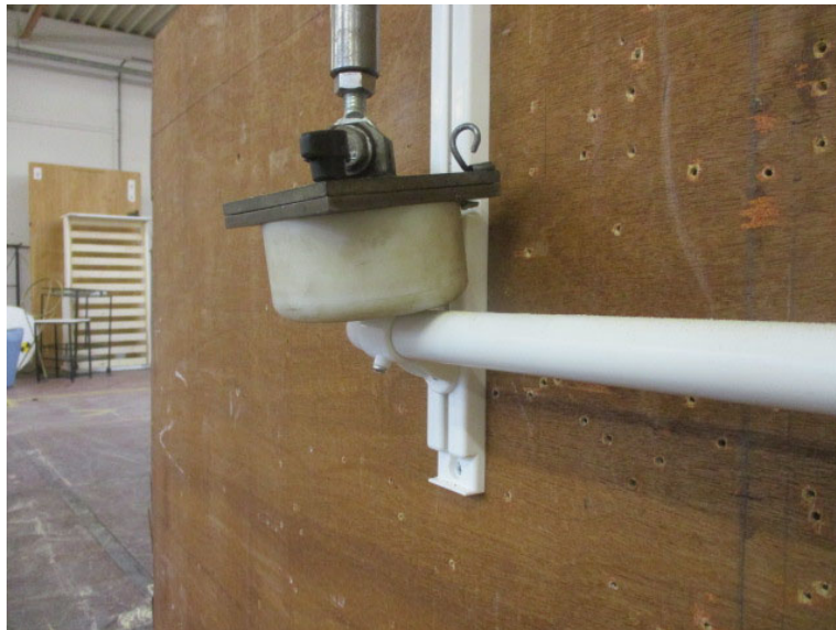
Photo 6: KiddieRail. Test 3 – Point Load application.
