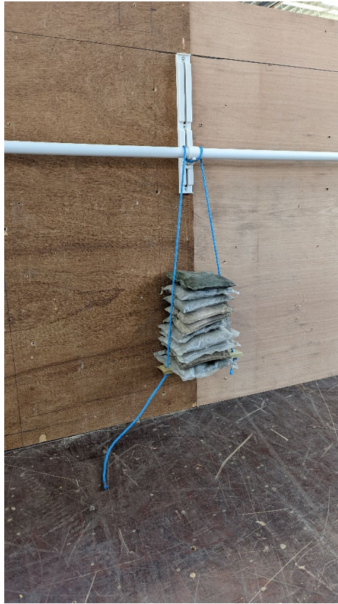
Photo 5: KiddieRail. Test 2 – 10Kg load x 48hrs.
