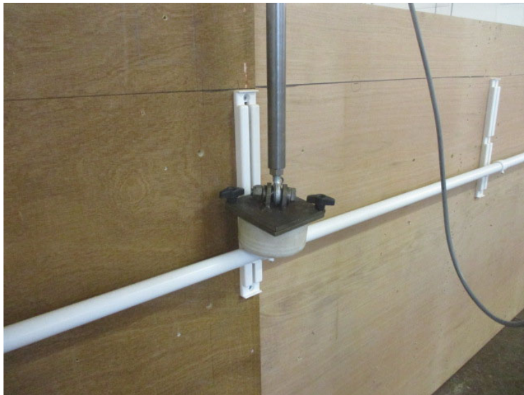
Photo 4: KiddieRail. Test 1 – Durability 14,600 cycles x 5Kg
